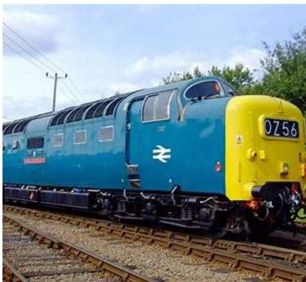
**After steam engines, diesel ones took over.** Firstly the Class 55 Deltics, of which 22 were built between 1961 and 1962, these could reach speeds of 100 m.p.h. These lasted until 1978 where a recorded speed was attained of 117 m.p.h. The last one to run was actually in 1981
